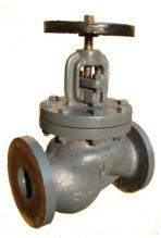
Bolted Bonnet is the most common design because there is practically no limitation on size. Multiple bolting permits equalized sealing pressure on the gasket against high pressure encountered in iron globe and angle valve applications.
